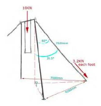
Net weight of rig – 99kg (full height) Max floor loading (excluding performers) – 40kg per leg Length of crane bar is 1.5m
